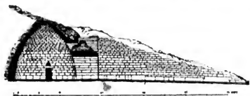
Fig 57.—Cupola tomb at Mycenæ—section (Baumeister.)
